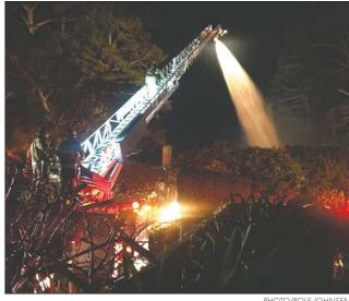
A water spout mounted on the top of a ladder truck allowed fire crews to douse the flames from above.
