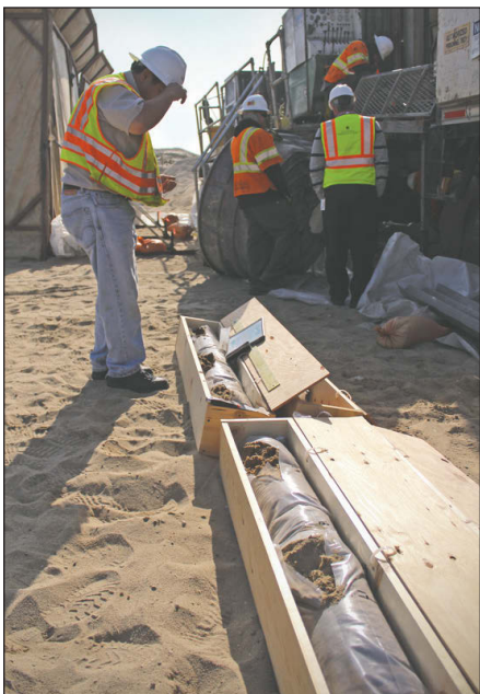
Borehole soil samples at the CEMEX property in Marina are being analyzed to determine if it will be the best site for wells for Cal Am's proposed desalination plant. So far, the answer is, "Yes."
