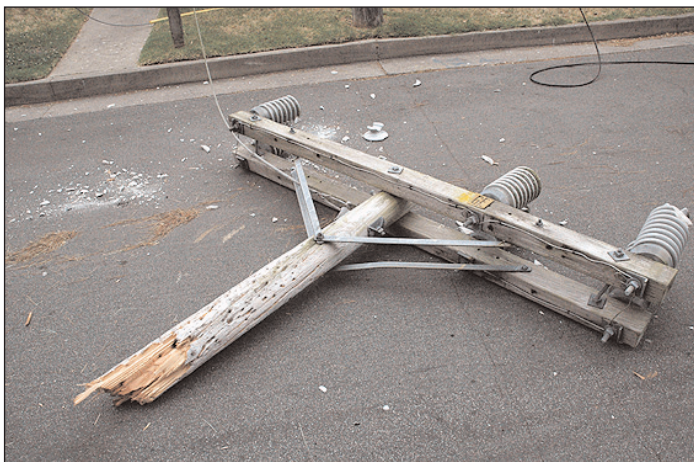
A towering Monterey pine (top) crushed two cars and a fence when it fell in Carmel Valley Monday afternoon, but it spared nearby houses and people. PG&E workers tried to figure out how to make repairs (left) after a 100-foot pine fell in Pacific Grove early Wednesday morning, decapitating several power poles when their wires were suddenly dragged down.
