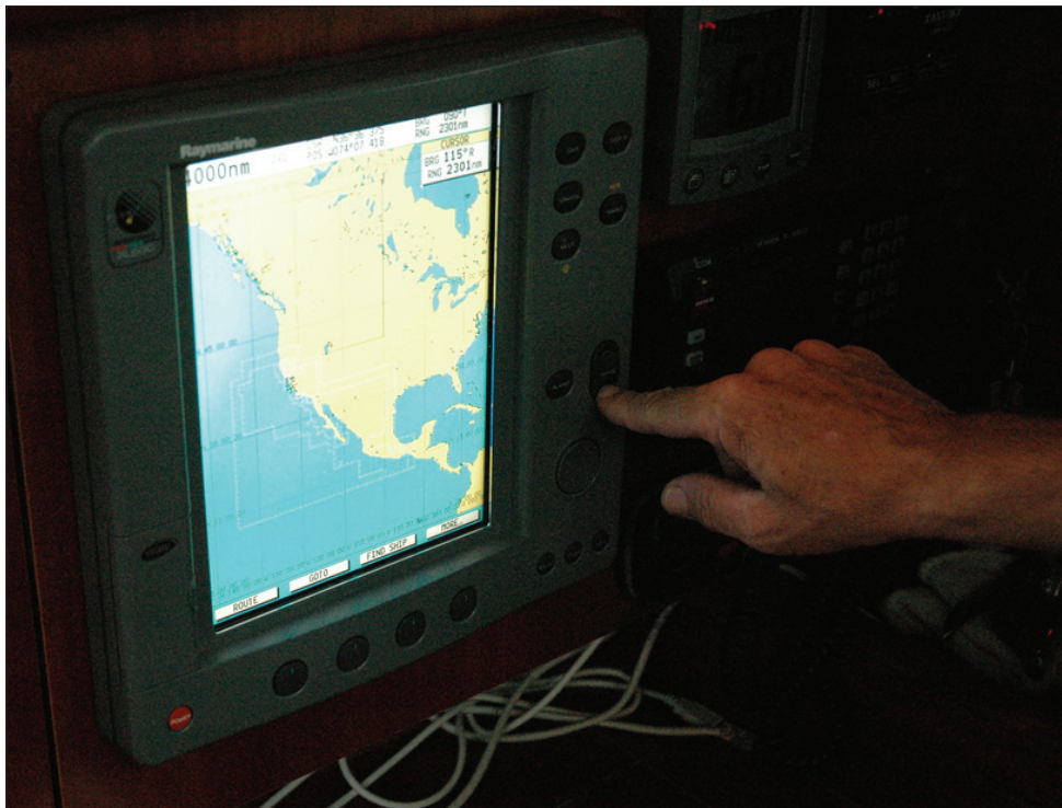
To make the Callisto seaworthy for such a lengthy trip, Humm installed a Raymarine navigational system, which includes a chart plotter tied into auto pilot, radar, and satellite navigational systems
